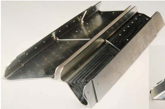
Intercostals machined on 5-Axis CNC using Aluminum Alloy 7050-T7451
